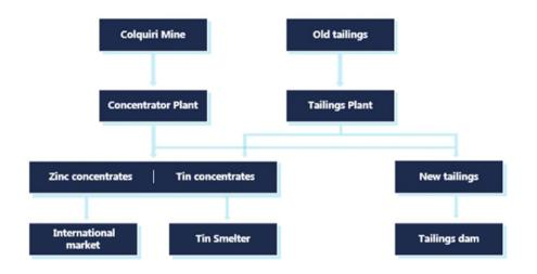
40. The Vinto Tin Smelter's operations consisted of purchasing tin concentrates from concentrate producers and traders, such as Colquiri, and smelting and extracting
