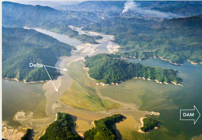
Sandy delta deposits advancing downstream in Porce II HEP reservoir, Colombia.
