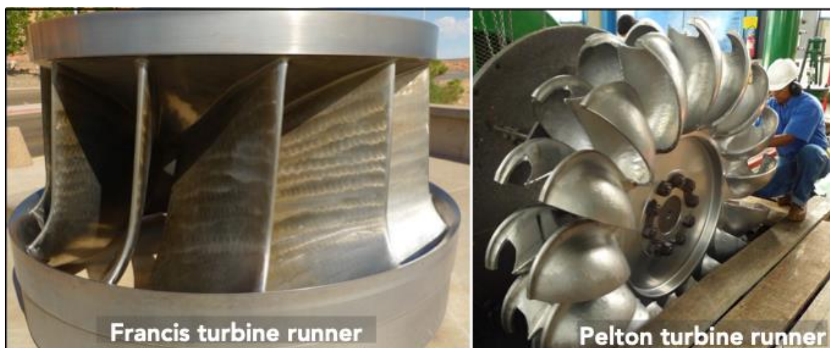
Figure 4.7 - Photographs of a Francis turbine runner (left) and a small Pelton turbine runner (right) 365
