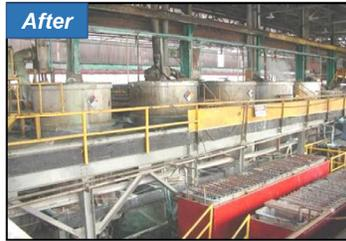
Copper sulfate cells to treat acidic solutions from copper refinery (c. 2004).
