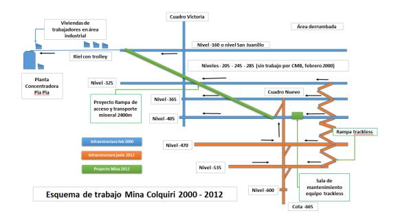
56. Work on the Main Ramp and underground infrastructure started in early 2012,<sup>95</sup> including civil work for the new warehouses and the acquisition of part of the materials to construct the improved underground infrastructure.<sup>96</sup>
