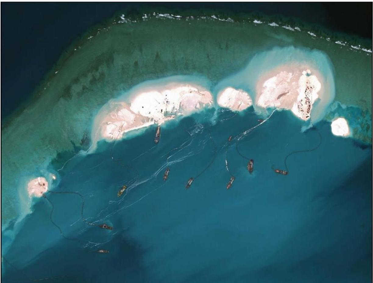
*Figure 17: Dredgers at work at Mischief Reef
