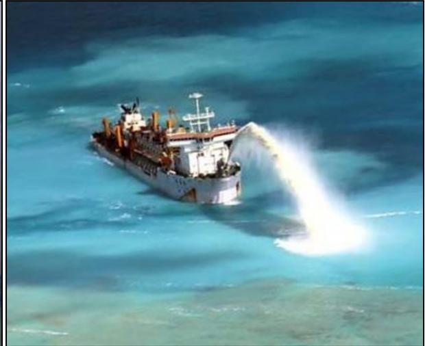
*Figure 16: Trailing Suction Hopper Dredge
