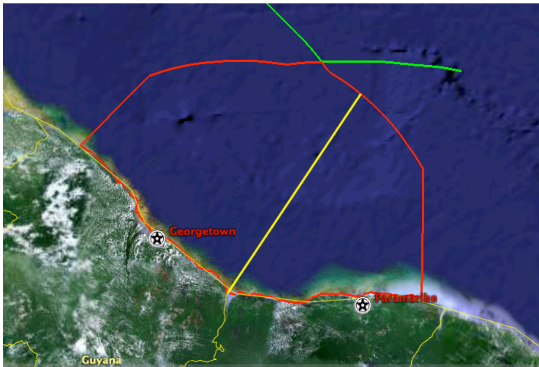
Figure 14. Division of the region shown in Figure 9 by the 34-degree line. The yellow line is a loxodrome with a bearing of 34 degrees. The green curves are extensions of the 200 nmi boundary.
