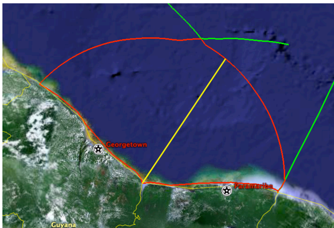
Figure 8. The division of the region in Figure 3 by the 34-degree line. The red curve outlines the entire region. The yellow line is a loxodrome with a bearing of 34 degrees. The green curves are extensions of the 200 nmi boundary and the Suriname – French Guyana equidistance line.
