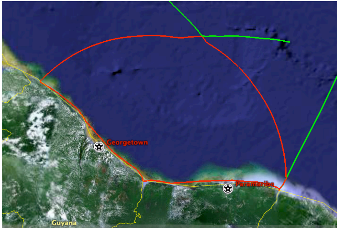
Figure 3. Region defined by the control point for each coast, the 200 nmi boundaries, and the Suriname – French Guyana equidistance line. The red curve outlines the entire region. The green curves are extensions of the 200 nmi boundary and the Suriname – French Guyana equidistance line.
